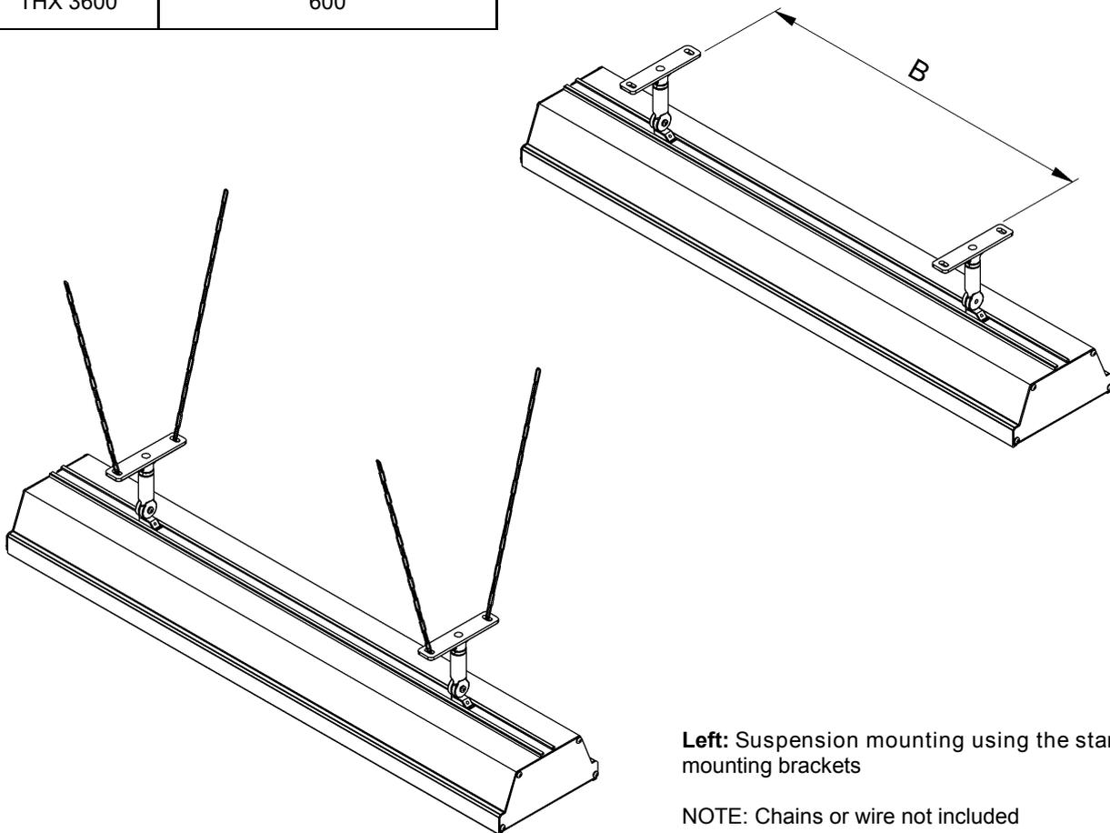
**Left:** Suspension mounting using the standard mounting brackets
