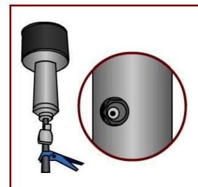
**1.** Screw the pipe and regulator assembly into the heater head. Point the adjustment screw on the regulator to the front of the heater.
