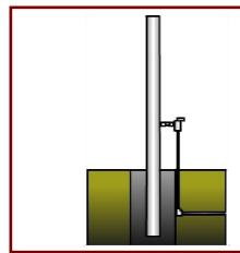
**3.** Concrete the pole into the ground to a depth of 450mm.
