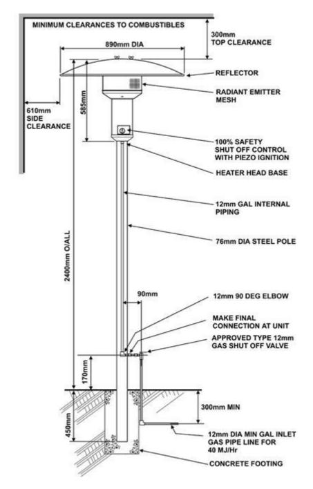
Overall height 2400mm. Overall width 890mm.
