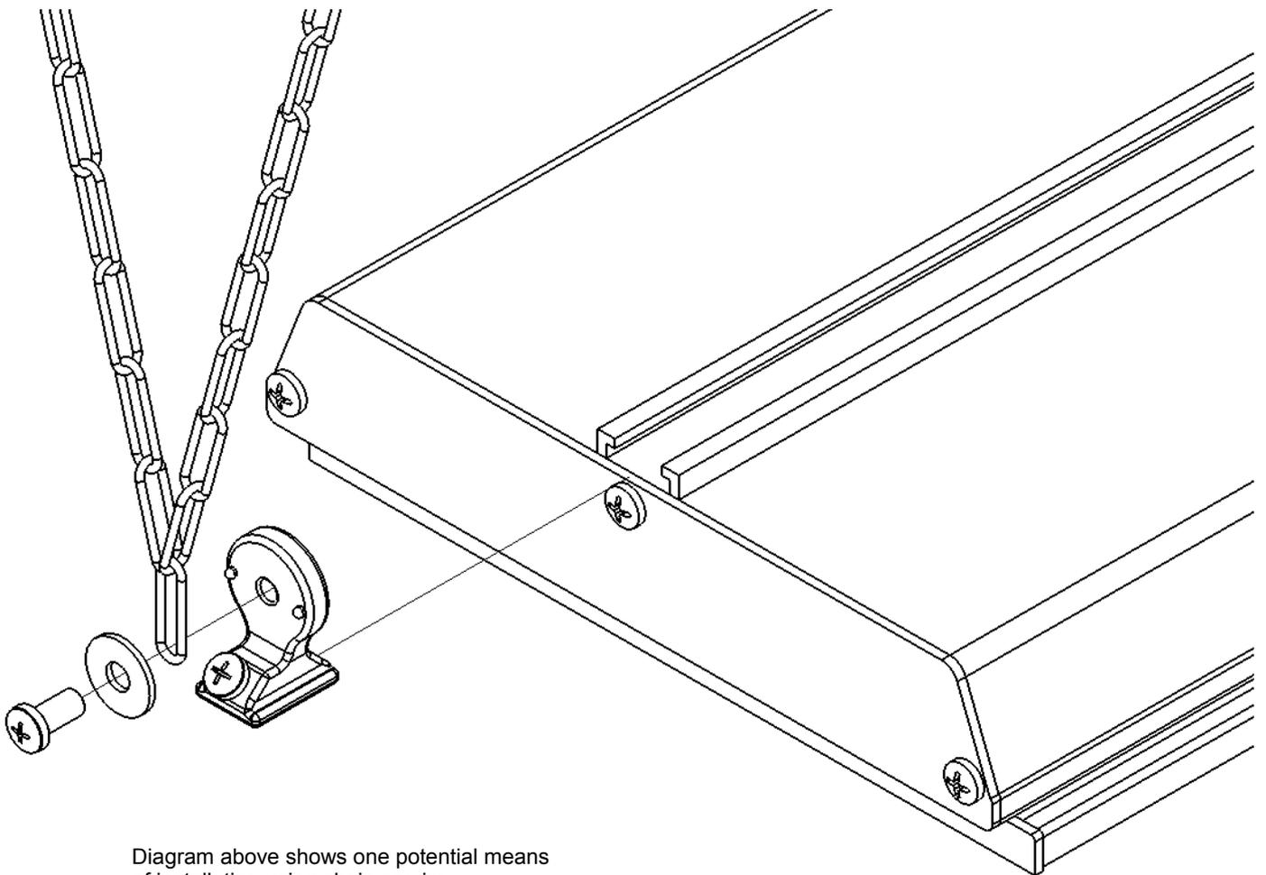
Diagram above shows one potential means of installation using chain or wire
