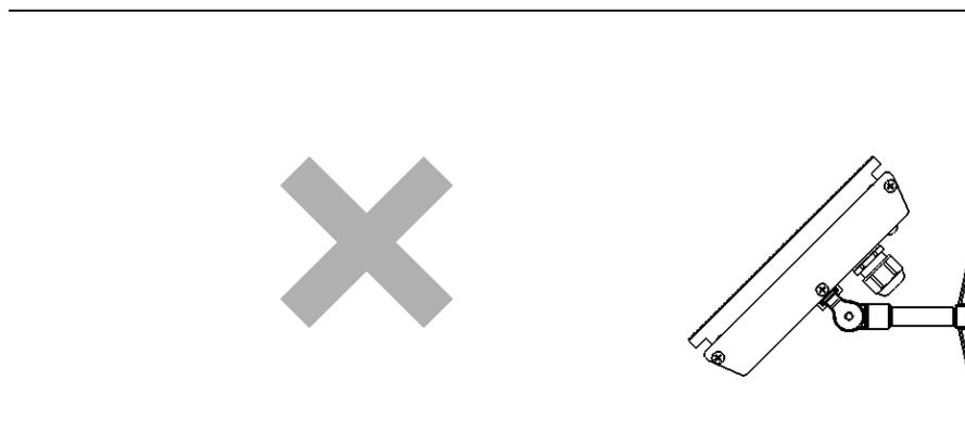
The heating surface must never be directed toward the ceiling
